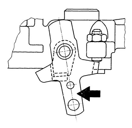
Mark control lever and shaft with respect to one another (arrows). Remove fastening screws for distributor—pump cover. Raise cover and press shaft inwards.
